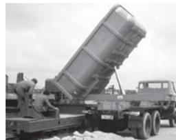
Michael also invented a 3 way tipper called the Revolver which was specially designed to tip its load to the side whilst still being driven forward. This was specifically used for laying the new concrete hard standing at Heathrow Terminal 4.
