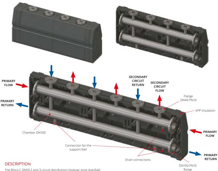
The Rhico C DN50 2 and 3 circuit distribution modular zone manifold is made with cylindrical flow and return tubes, completely separated and insulated. The main connections to the heat generator and to the secondary circuit are flanged.
